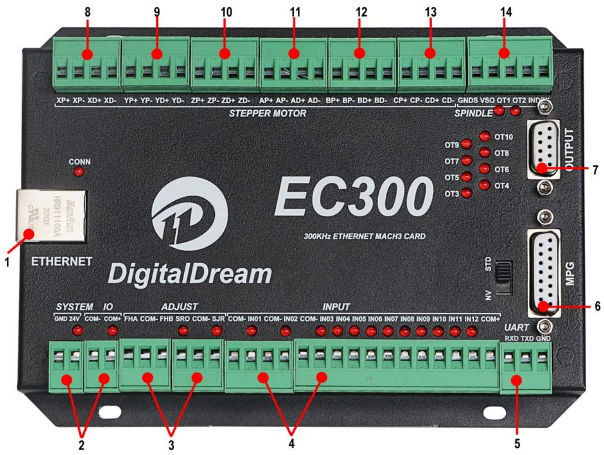
Figure2-1. Product wiring section and interface summary
